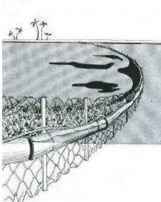
Fixed oil barrier constructed with straw bales and wire netting nailed to wooden stakes.
