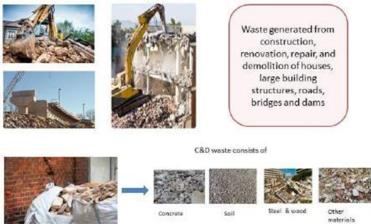
Figure 14 Components of C&D waste
