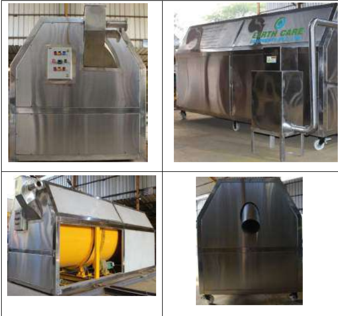
Figure 17: Typical Organic Waste Converter
