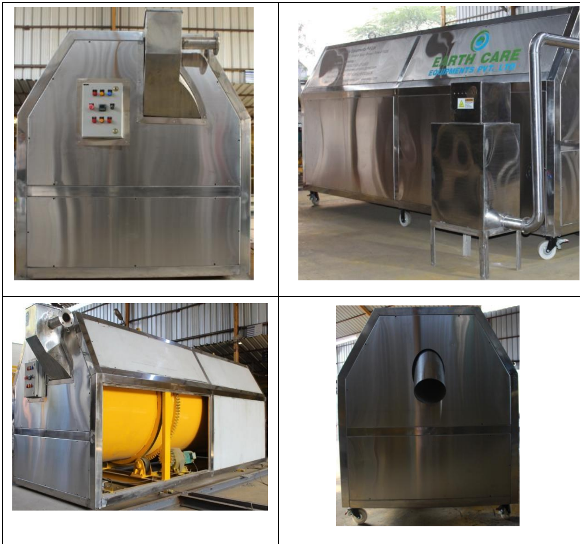
Figure 17: Typical Organic Waste Converter
