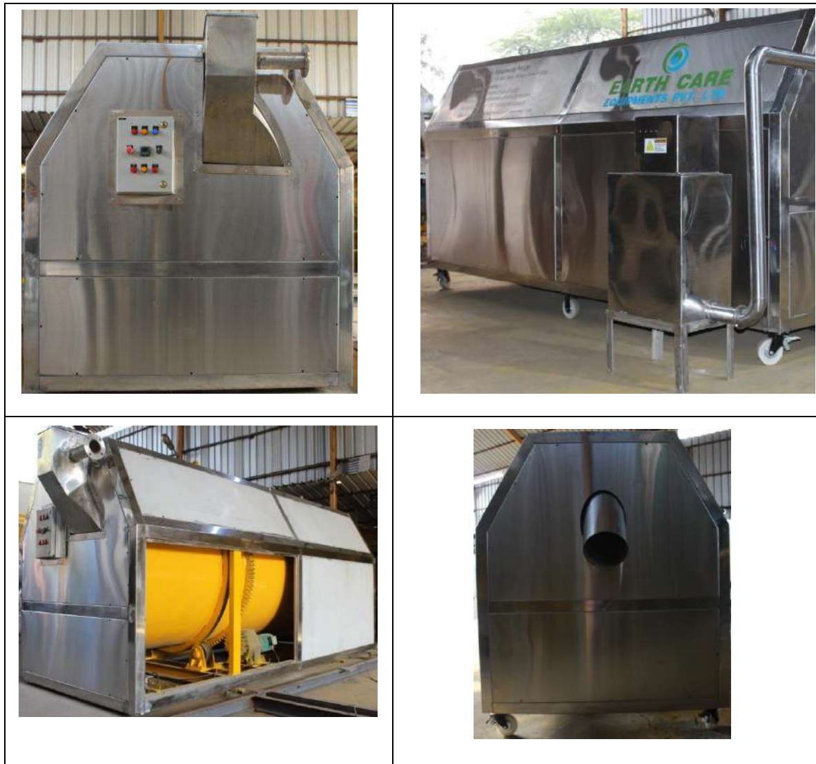
Figure 17: Typical Organic Waste Converter
